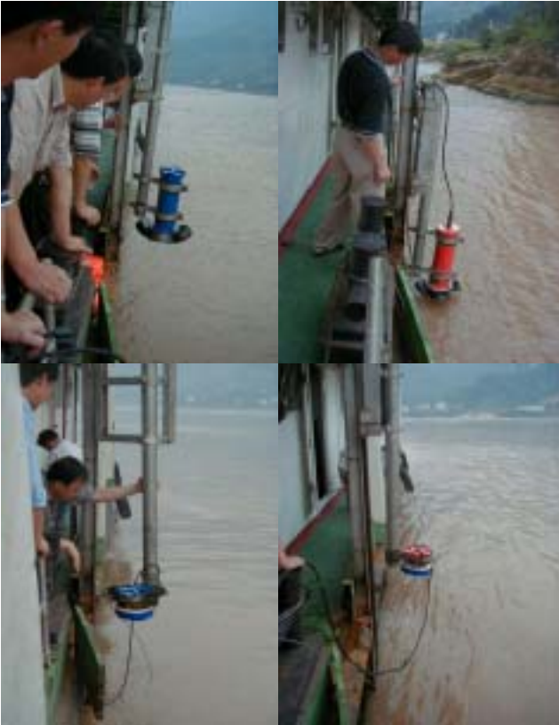
Figure 3 ADCPs used in the tests. Top left: 150 kHz WH ADCP; Top right: 300 kHz BB ADCP; Bottom left: 300 kHz WH Minitor ADCP; Bottom right: 600 kHz WH Rio Grande ADCP
