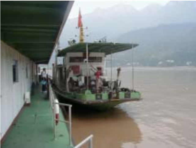
Figure 1 A steel-hulled survey vessel used in Yangtze River ADCP discharge measurements
