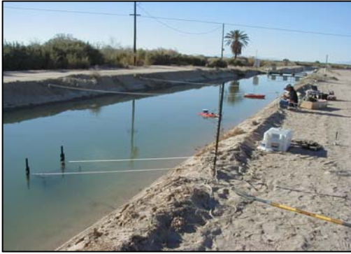
Figure 2 StreamPro ADCP attached to a pulley system 57 meters (187 feet) upstream Trifolium 13 Check structure; ChannelMaster H-ADCP mounted 7.6 meters (25 feet) upstream the pulley.
